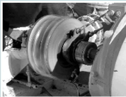
The MagnaDrive in action (left). The magnetic coupler device spins rapidly, controlling the engine RPM and adjusting pump flow.
